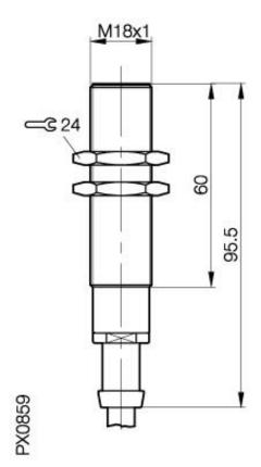
Inductive Sensors BES 516-105-SA2-05 M18x1 x 95.5 Complementary Sn=5mm shielded temperature rated
